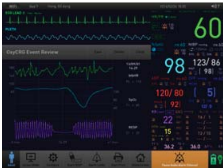
OXI-CRG ECG + Spo2 + respiration combined parameter for Neonatal breathing sufficiency & brain maturity
