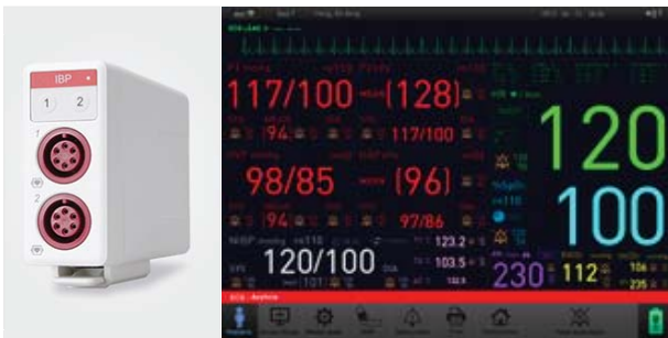
Dual IBP module 2 or 4CH IBP Selectable label (ABP, ART, AO, UAP, P, PAP, ICP, RAP, LAP, UVP)
